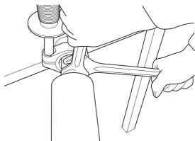
Before the machine is started, carefully check that the new bit is firmly attached.
