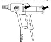
• Use compressed air to periodically clean the motor. Remove the inspection cover and clean the cover.
